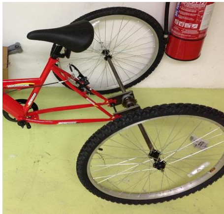
Figure 5: Application of shaft on the rear wheels to the main frame.
