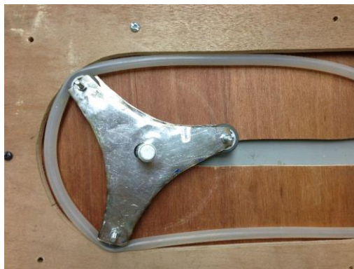
Figure 6: Peristaltic pump made up of metal plate and rollers.
